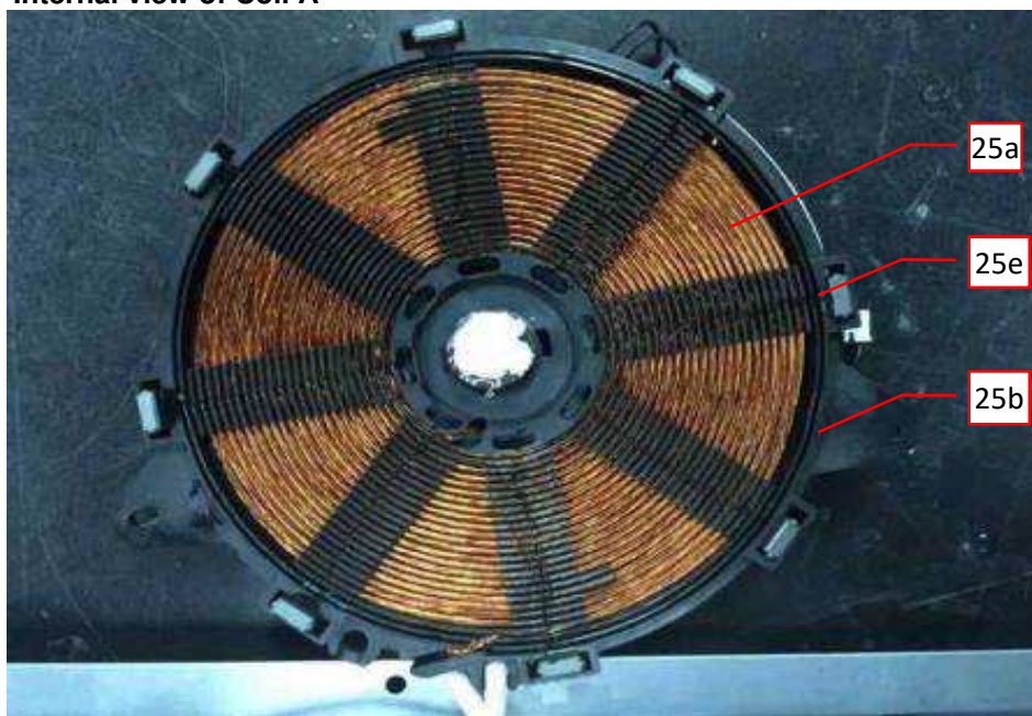
Photo 49 - Internal view of Coil A
