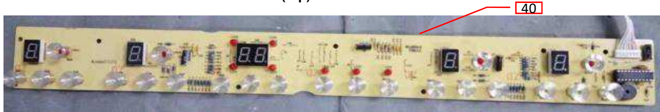
Photo 70 - Internal view of C74E Control 05 (top)
