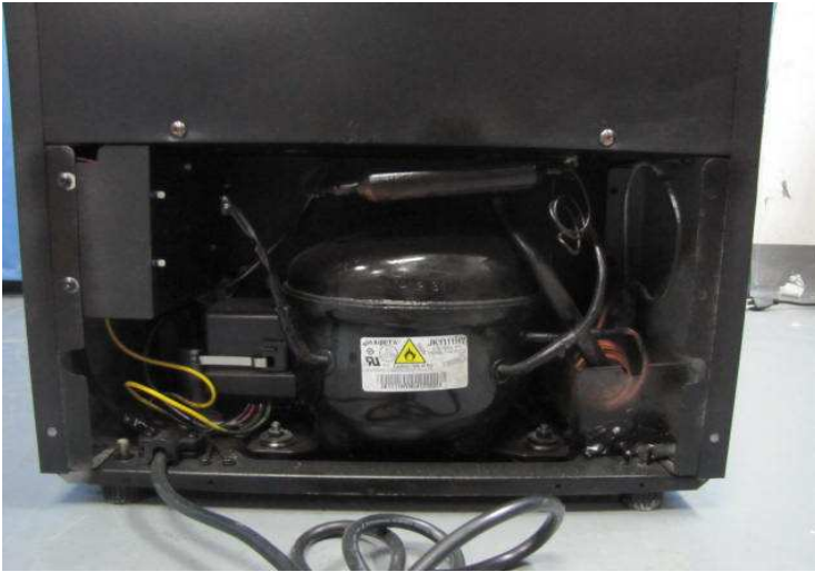
Photo 19 - Compressor compartment for CWC-150 series
