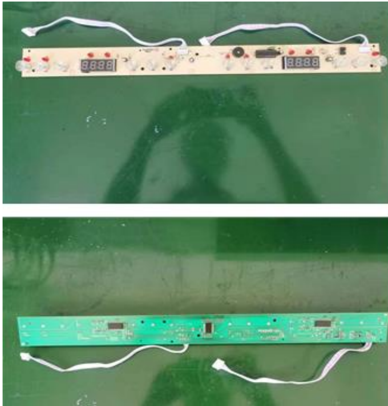
Photo 40 - Control PWB view for model C18E-DEH02.
