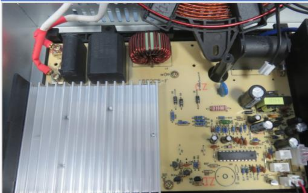
Photo 30 - Alternative FILTER BOARD for models C18E-DDS01, C18E-DES01
