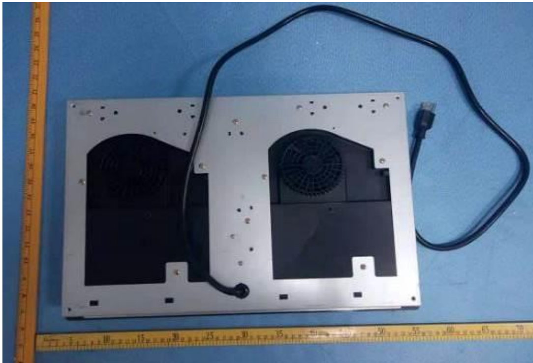
Photo 37 - Alternative construction for metal enclosure of models C18E-DDH02, C18E-DEH02
