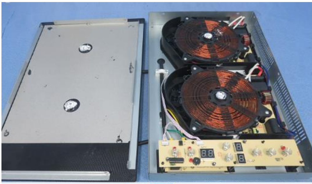
Photo 36 - Alternative construction for metal enclosure of models C18E-DDS01, C18E-DES01
