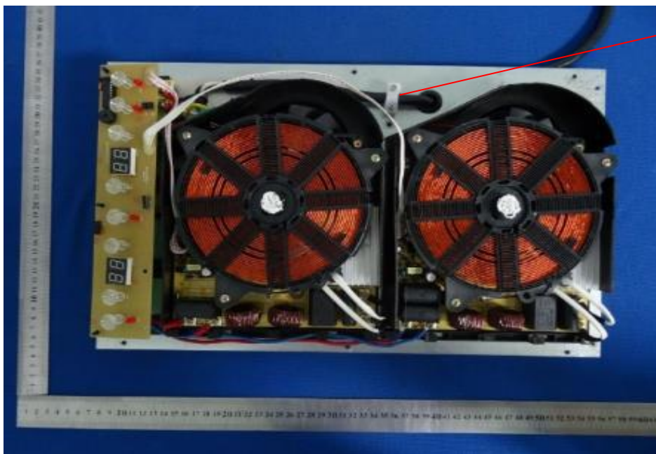
Photo 11 - Internal view for models C18E-DDS01, C18E-DES01.
