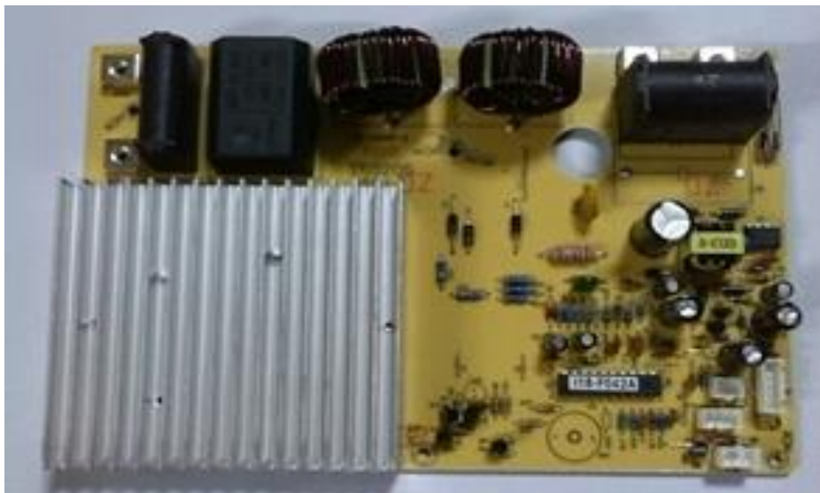
Photo 26 - Power PWB view - for 1300W hotplate
