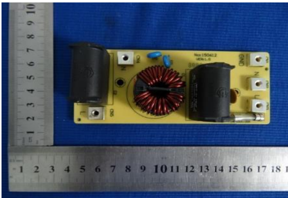
Photo 20 - Filter PWB view - for C18E-DDH02, C18E-DEH02
