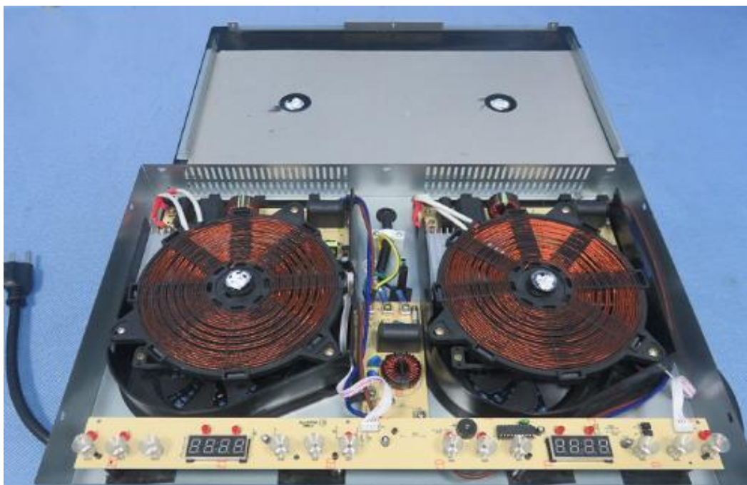
Photo 34 -Internal view for models C18E-DDH02, C18E-DEH02
