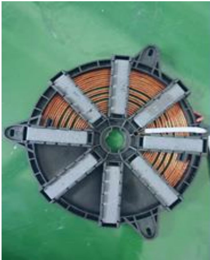
Photo 34 -Internal view for models C18E-DDH02, C18E-DEH02
