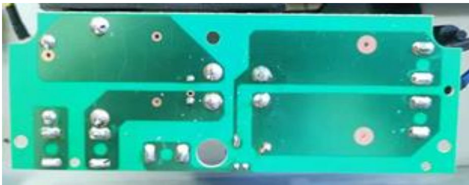
Photo 44 - Alternative FILTER BOARD bottom View for models C18E-DDH02, C18E-DEH02, MD-2B
